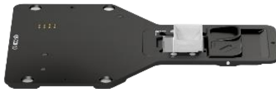
Figure 9: Chip Carrier Base (CCB) with the Chip Carrier (CC) and QuChip mounted on top
