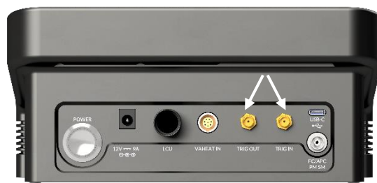
Figure 28: The SMA cables for the trigger IN and Out are connected to the QUSCITE control unit back panel.
