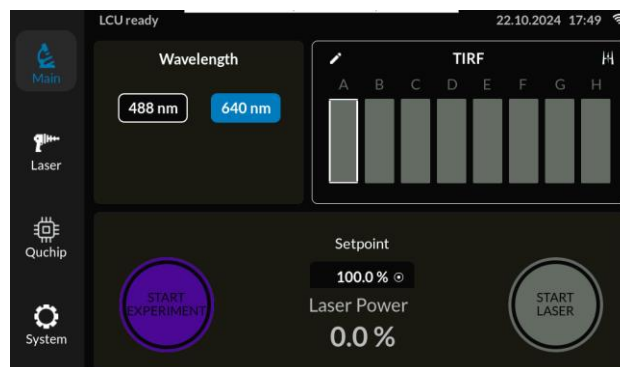
Figure 19: On the main menu you can select the waveguide on the top right side of the screen
